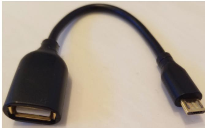
Notice the "female" connection on the left side view. This is where the "male" connection on the bar code scanner will go. There is no electronics in these adapters, they are simply reducing the connection from the large USB to the small micro plug, so they are rather inexpensive. Here's our total setup:
